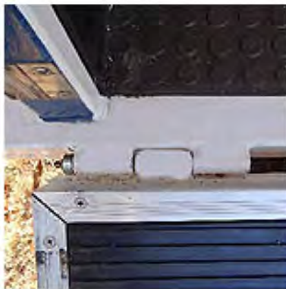
All hinges greasable - drop down ramp
