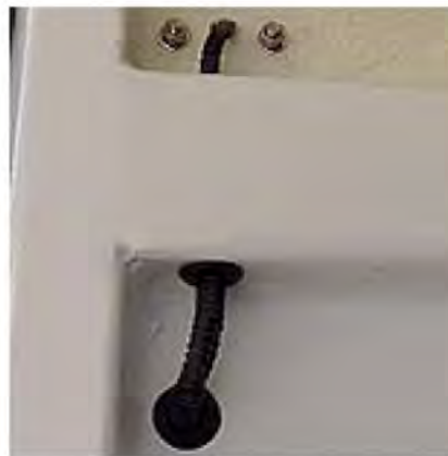
All wires run through chassis fully grommited
